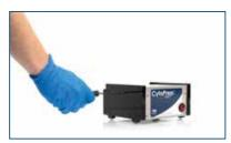
If there is debris visible, or the fans are not running well, remove the side panels using a 3mm hex wrench.
